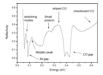
Fig. 1. The assignment of the MIR reflectivity features to several phases. Reproduced from [11].
